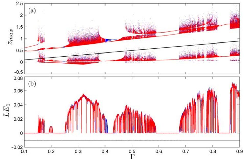
Fig. 4. (a) Bifurcation diagrams for local maxima of  $z$  versus the parameter  $\Gamma \in [0.1, 0.9]$  and (b) variation of the corresponding largest Lyapunov exponents for system (1) with  $\mu = 0.08$  and  $\nu = 0.1$ .
