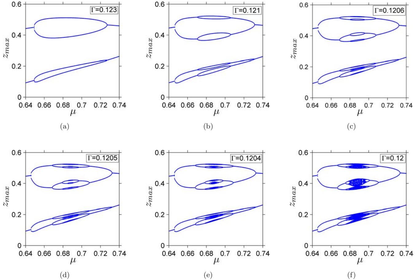
Fig. 9. Onset of chaos via period-bubbling cascades: (a) period-4 bubble at  $\Gamma = 0.123$ , (b) period-8 bubble at  $\Gamma = 0.121$ , (c) period-16 bubbles at  $\Gamma = 0.1206$ , (d) period-32 bubbles at  $\Gamma = 0.1205$ , (e) and (f) chaos delimited on both sides by period-doubling cascades at  $\Gamma = 0.1204$  and  $\Gamma = 0.12$ , respectively.
