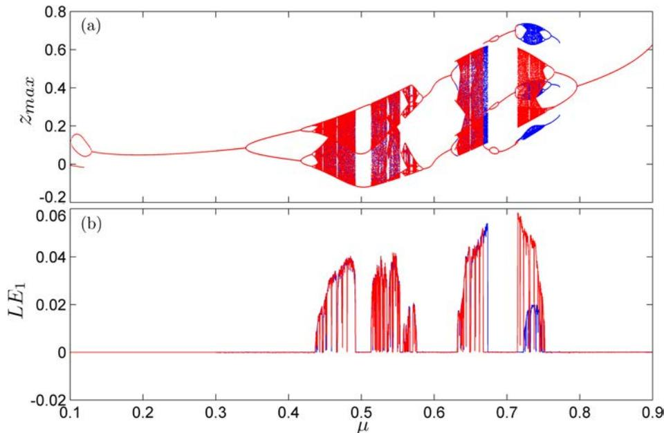
Fig. 1. (a) Bifurcation diagrams for local maxima of  $z$  versus the parameter  $\mu \in (0.1, 0.9]$  and (b) variation of the corresponding largest Lyapunov exponents for system (1) with  $\nu = \Gamma = 0.1$ .
