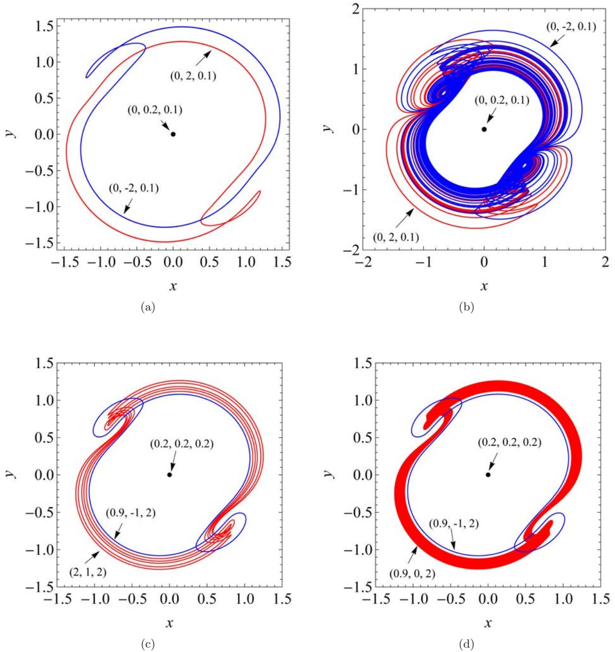
Fig. 6. Phase portraits (projected onto the  $xy$ -plane) of the coexisting multiple attractors of system (1) for different values of  $\Gamma$  with  $\nu = 0.1$  and  $\mu = 0.08$ : (a)  $\Gamma = 0.62$ , (b)  $\Gamma = 0.30$ , (c)  $\Gamma = 0.405$  and (d)  $\Gamma = 0.406$ .
