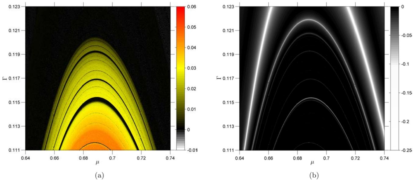
Fig. 8. Variation of the two leading Lyapunov exponents  $LE_{1,2}$  ( $LE_1 \geq LE_2$ ) [(a)  $LE_1$  and (b)  $LE_2$ ] of system (1) in the biparameter space  $(\mu, \Gamma) \in [0.64, 0.74] \times [0.111, 0.123]$  with  $\nu = 0.1$ . The color bars represent the color codes of the numerical values of the Lyapunov exponents.
