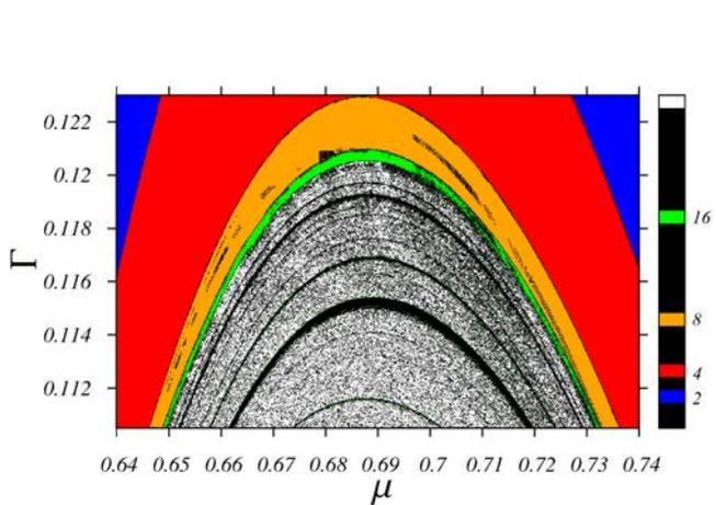
Fig. 10.  $\mu$  versus  $\Gamma$  parametric diagram in the occurrence of the period-bubbling. The color bar represents the periods of the periodic regions.
